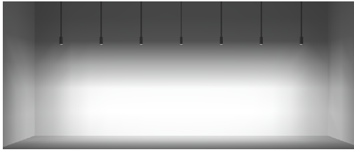
8FT MOUNTING HEIGHT 36" SETBACK / 48" ON CENTER SPACING
