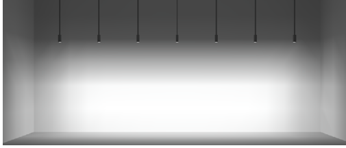
8FT MOUNTING HEIGHT 36" SETBACK / 48" ON CENTER SPACING
