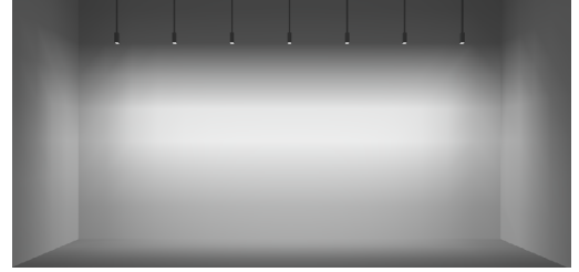
12FT MOUNTING HEIGHT 36" SETBACK / 48" ON CENTER SPACING
