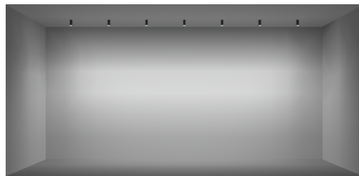
12FT CEILING 36" SETBACK / 48" ON CENTER SPACING
