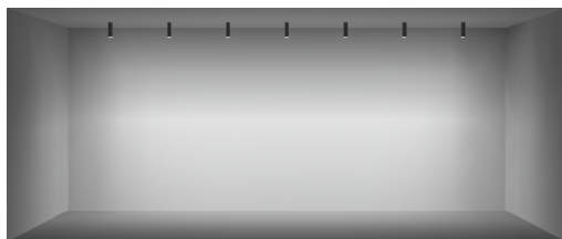
8FT CEILING 36" SETBACK / 48" ON CENTER SPACING
