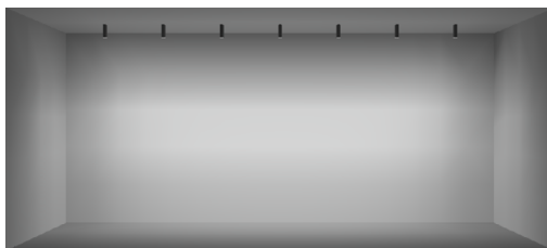
10FT CEILING 36" SETBACK / 48" ON CENTER SPACING
