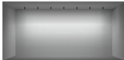
12FT CEILING 36" SETBACK / 48" ON CENTER SPACING
